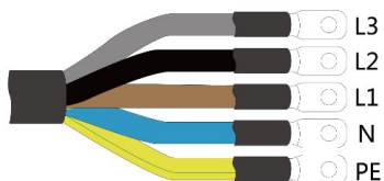
figure 2-6 Cable connection terminal
